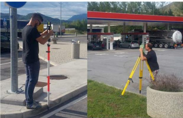
Figure 3. Validation survey with total station
